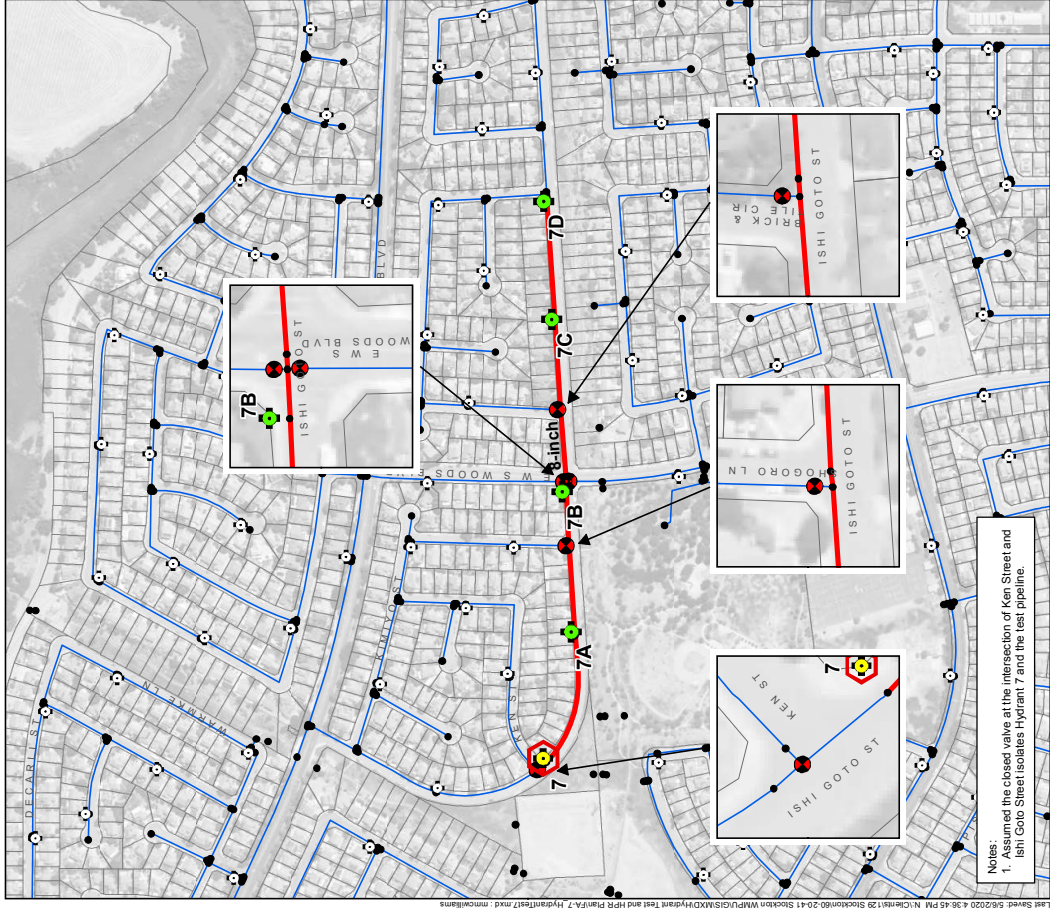
Figure A-7 Test 7 (8-inch PVC - 1990s) City of Stockton Water Master Plan Update
